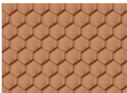
Pose double recouvrement pointe
